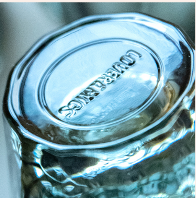
Debossed Embed in the moulds
